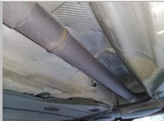
Engine to silencer pipe
