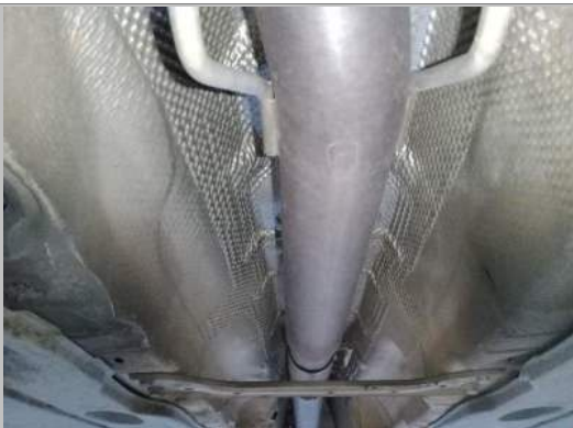
Engine to silencer pipe
