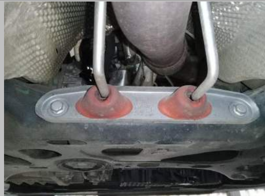
Engine to silencer pipe
