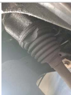
CV Joint(s) Boot(s) Front Left (inner/outer)
