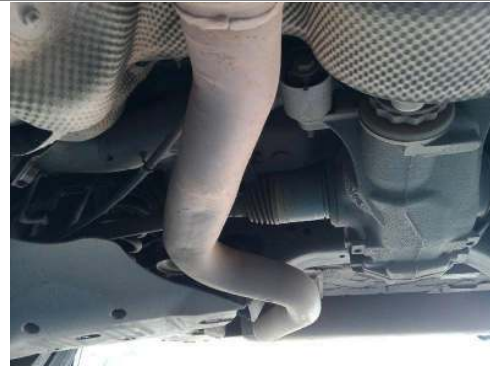
Engine to silencer pipe
