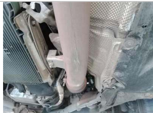
Engine to silencer pipe
