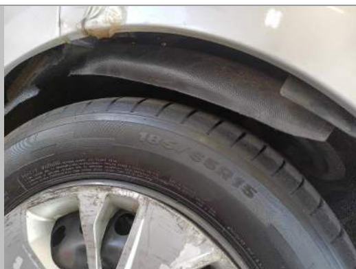
LEFT FRONT FENDER LINER LOOSE
