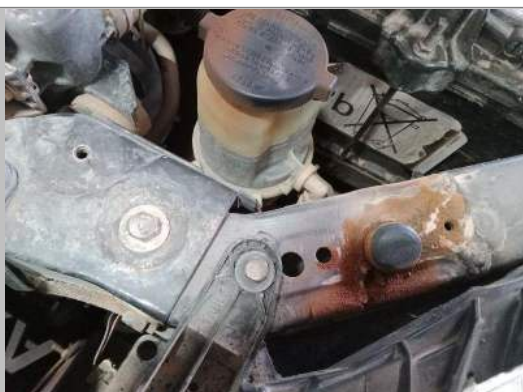
Bonnet slam plate (Shock tower/ Inner tray)
