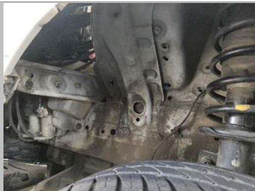
L/F fender liner missing
