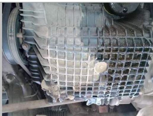
Engine oil sump
