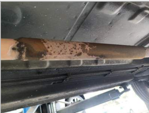
Engine to silencer pipe
