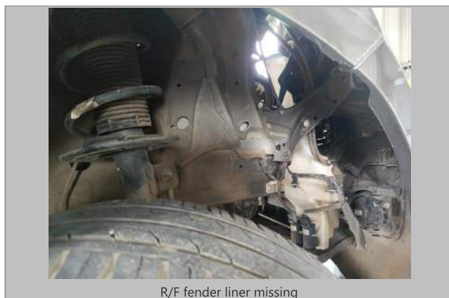
R/F fender liner missing
