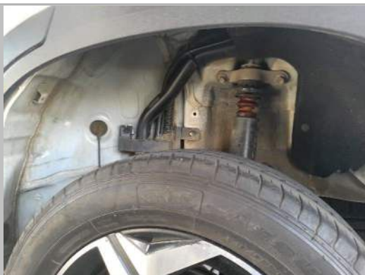
L/R fender liner missing
