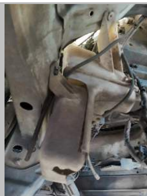
Window washer reservoir damage
