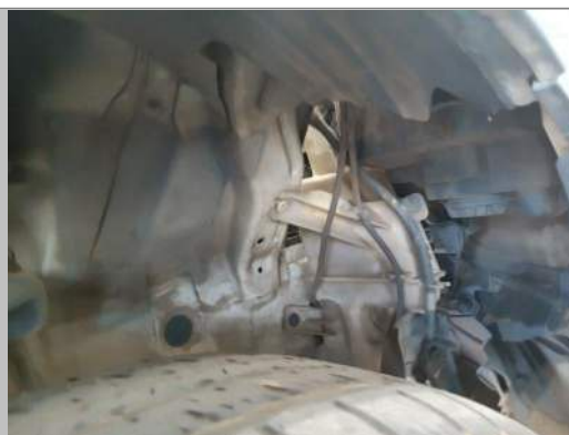
R/F fender liner missing
