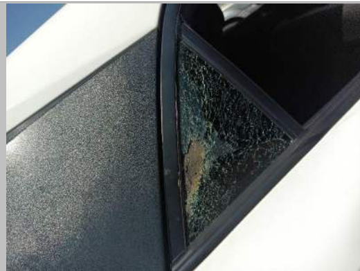
R/R window broken
