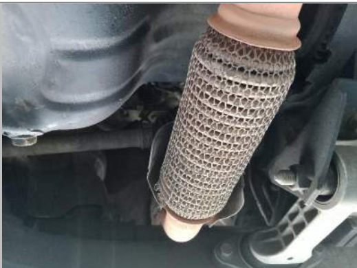
Engine to silencer pipe
