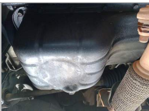
Engine oil sump
