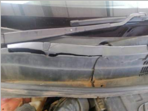
Wiper valance grill damage
