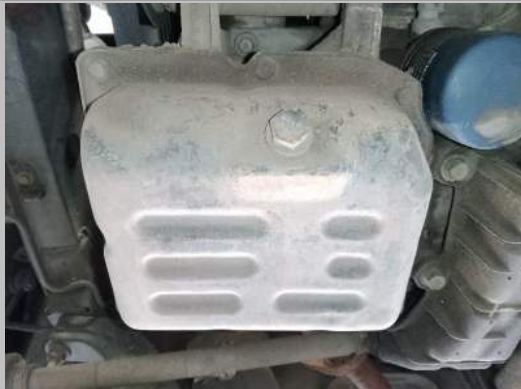
Engine oil sump
