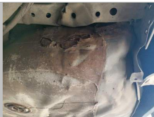
Sparewheel well signs of weldi
