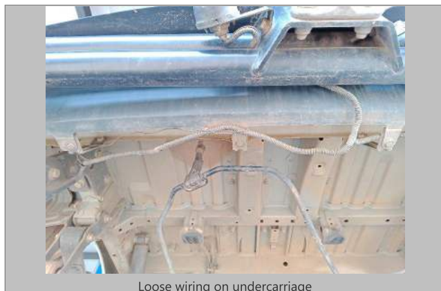
Loose wiring on undercarriage
