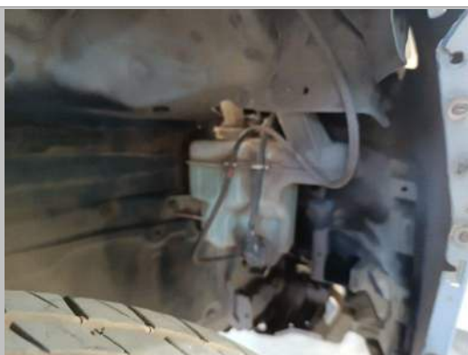
R/F fender liner missing
