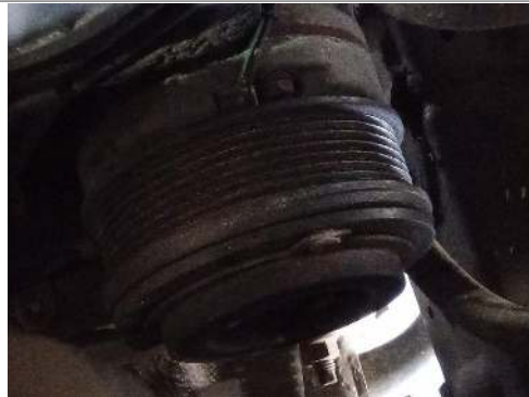
Air conditioner pump
