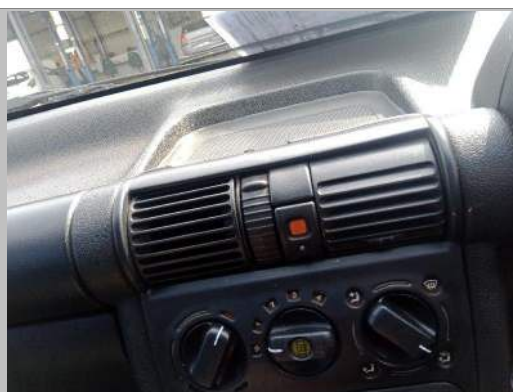
Central Air Vent
