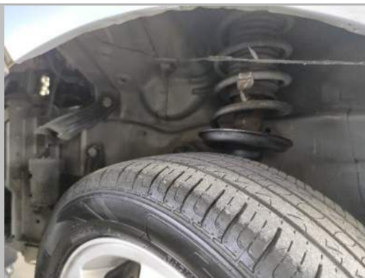
L/F fender liner missing
