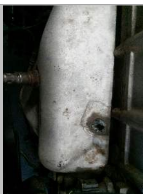
Engine heat shield damage
