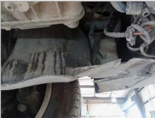
Front Fender Left / Inner Tray
