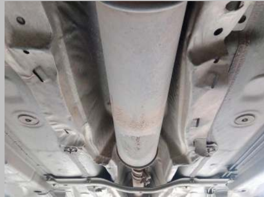
Engine to silencer pipe
