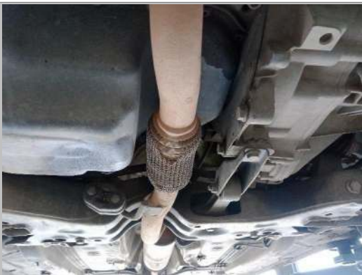
Engine to silencer pipe
