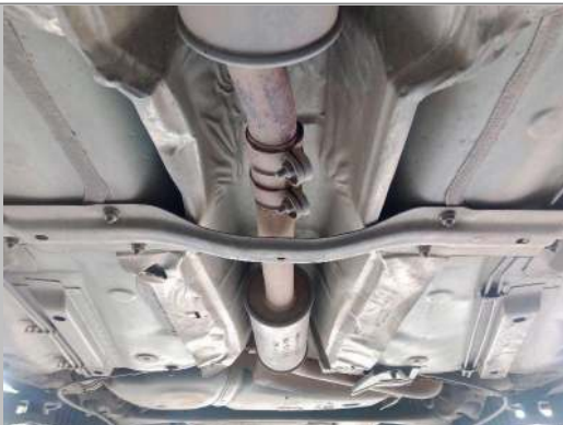
Engine to silencer pipe
