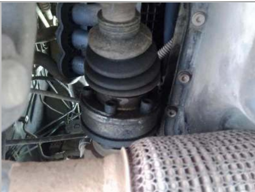
CV Joint(s) Front Right (inner/outer)
