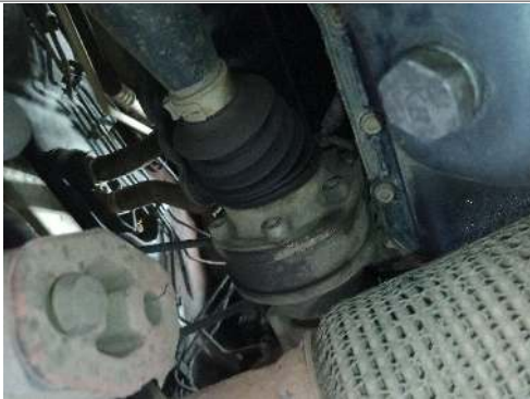
CV Joint(s) Front Right (inner/outer)
