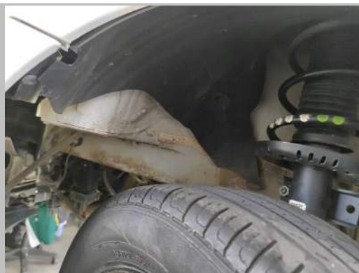
L/F fender liner missing
