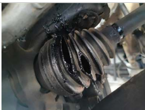
CV Joint(s) Boot(s) Front Left (inner/outer)
