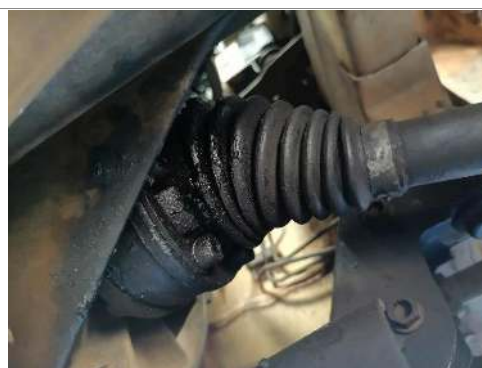
CV Joint(s) Boot(s) Front Left (inner/outer)
