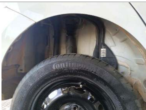
R/R fender liner missing
