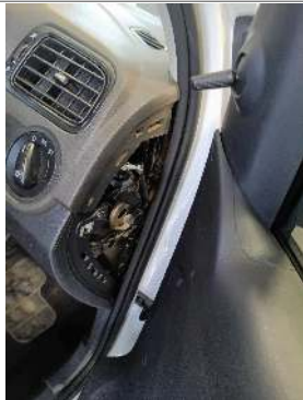
Sider cover missing
