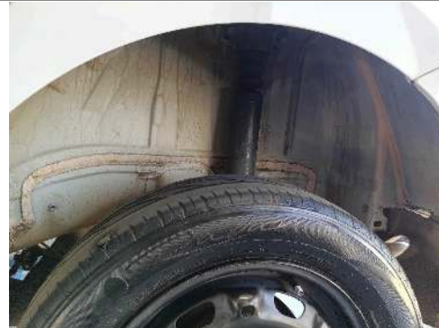
L/R fender liner missing
