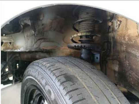
L/F fender liner missing
