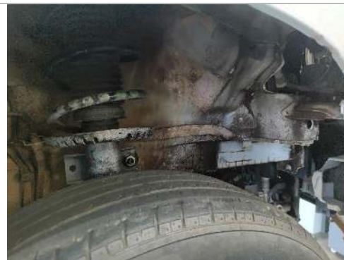
R/F fender liner missing
