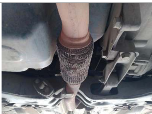
Engine to silencer pipe
