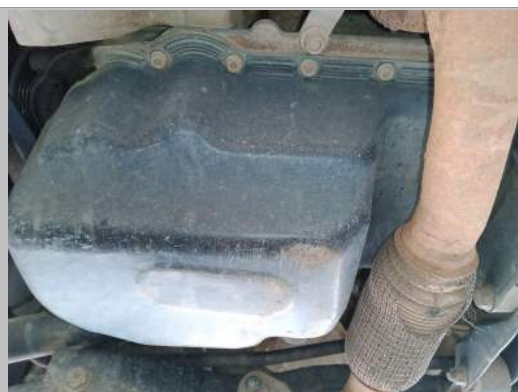
ENGINE OIL SUMP
